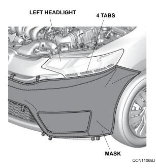
11. Attach the eight hooks to the inside edge of the lower grille opening and front grille opening.
